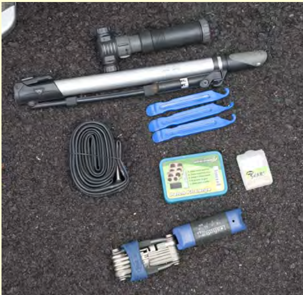
Top: two kinds of tire pumps. The smaller one fits in a seat bag and works on both Presta and Schrader valves. The larger frame pump is for Presta only, but has a built-in gauge and is easier to use. Middle: spare inner tube, set of tire levers and both kinds of patch kits. Bottom: a bicycle multitool, and an Allen wrench set. You should carry one or the other.
