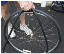
Starting with the valve stem, push the tube into the tire
