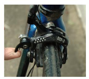
**Now you can remount the wheel** on the bike. You may find that while it was easy to remove the wheel when the tire was flat, it may be hard or even impossible to put back on even partially inflated.
