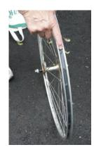
In the unlikely event that the puncture is on the inside of the tube, you should remove the tire and check the rim for protruding spoke ends. On the road, there is not much you can do about one of these except cover it with a tire patch and ride home. You might need to get the wheel repaired, or at least retaped.
