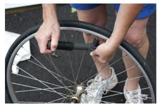
**Pump the tire** until it is firm enough to hold its shape when pressed with a finger, but not until it is hard enough to ride on. Then check to be sure that it is seated properly on the rim and that the tube isn't pinched between the tire and rim.
