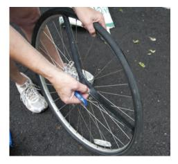
**Pull the inner tube from the tire.** You may have to undo a small nut from the valve stem.
