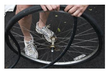
Push the tire back onto the rim using your thumbs. DO NOT pry it on with the tire levers!
