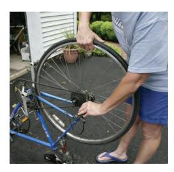
Turn the bike upsidedown and remove the wheel. Most modern bikes have quick release levers.
